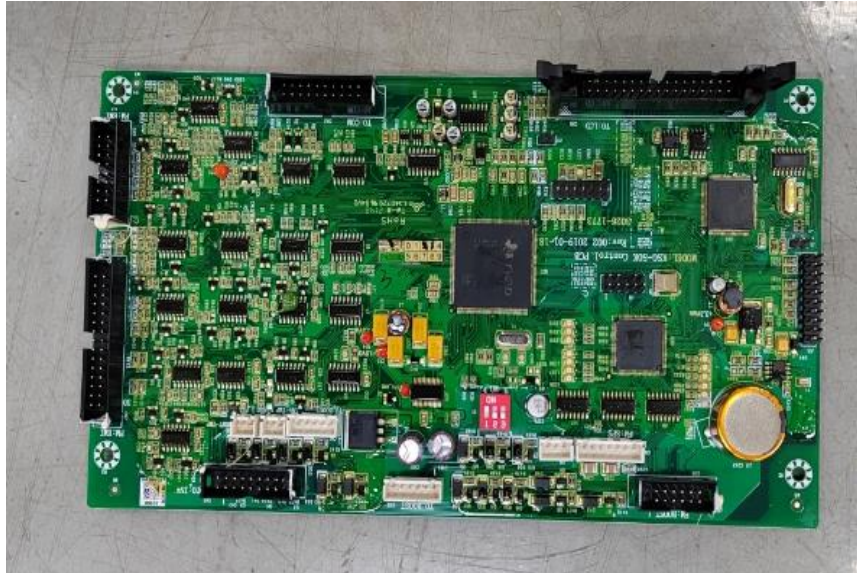
Figure 9. Front view of Control board (OCIP50-TL3-M3-OD-OL/FL)
