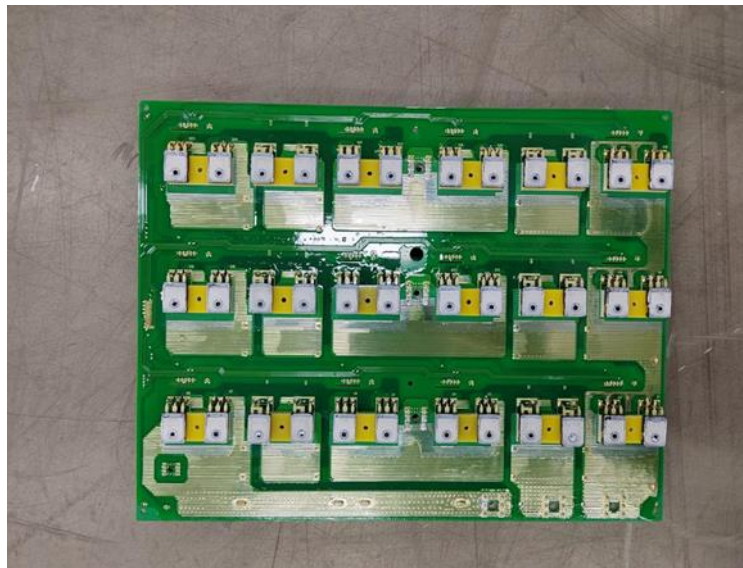
Figure 12. Back view of INV board
