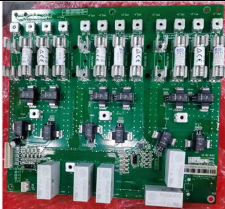
Figure 27. Front view of I03 board (OCIP50-TL3-M3-OD-OL,FL)
