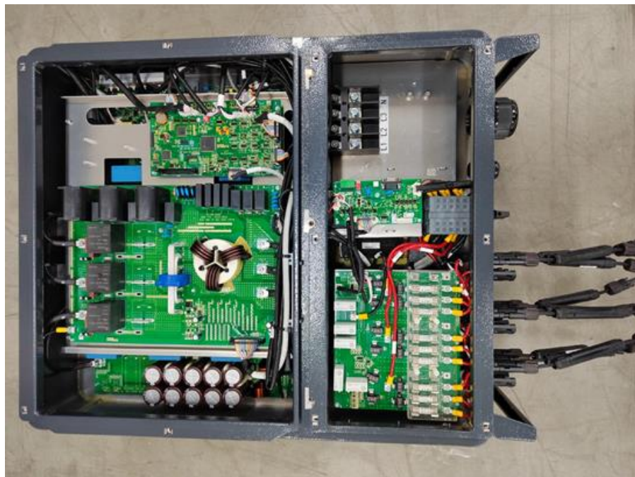
Figure 6. Internal view of model (OCIP50-TL3-M3-OD-OL, FL)
