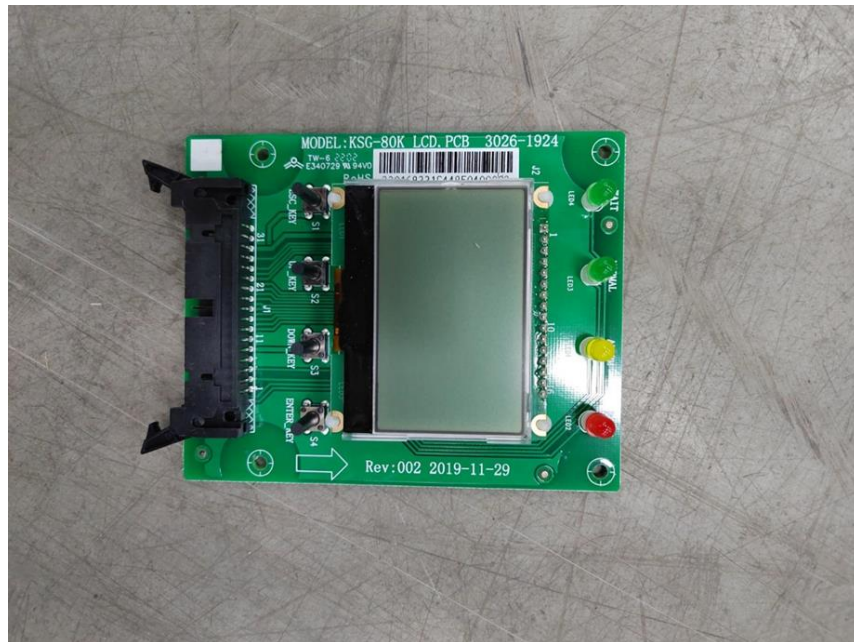
Figure 29.Front view of LCD board
