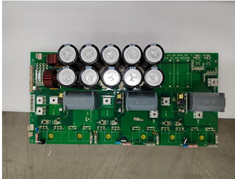
Figure 13. Front view of BOOST board
